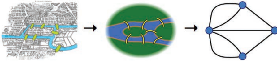
Figure 2 Representation of the Königsberg bridges problem as a graph problem, with an intermediate step in which the topology of the city has been simplified [12, 21].
